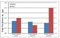
By using the blade material which differs to the inside (moving blade = Stainless Alloy) and outside (still blade = Cobalt Base Alloy CBA-12), the edge will not nick so easily.
