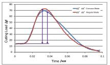
The new Concave Cobalt scissors will cut hair very well with less effort, because the cutting load is lower than existing scissors.
